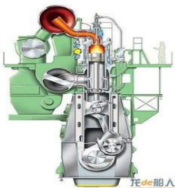
14K98ME-C – the most powerful engine ordered: Bore: 980 mm Stroke: 2,660 mm Speed: 104 r/min Output: 84,280 kW Fuel cons: 346 ton/day Weight: 2,219 ton Height: 14.6 m Length: 29 m
