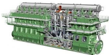
14K98ME-C – the most powerful engine ordered: Bore: 980 mm Stroke: 2,660 mm Speed: 104 r/min Output: 84,280 kW Fuel cons: 346 ton/day Weight: 2,219 ton Height: 14.6 m Length: 29 m
